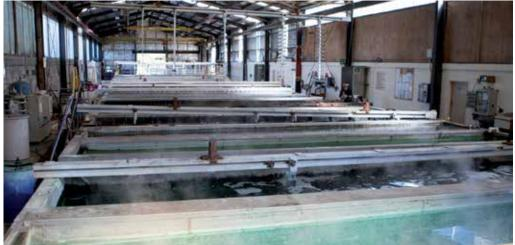
Anodising is a durable and hard wearing finish offering maximum protection in harsh environments. A range of colours and micron (7-25 $\mu$ m) finishes are offered to ensure you achieve the desired look.
